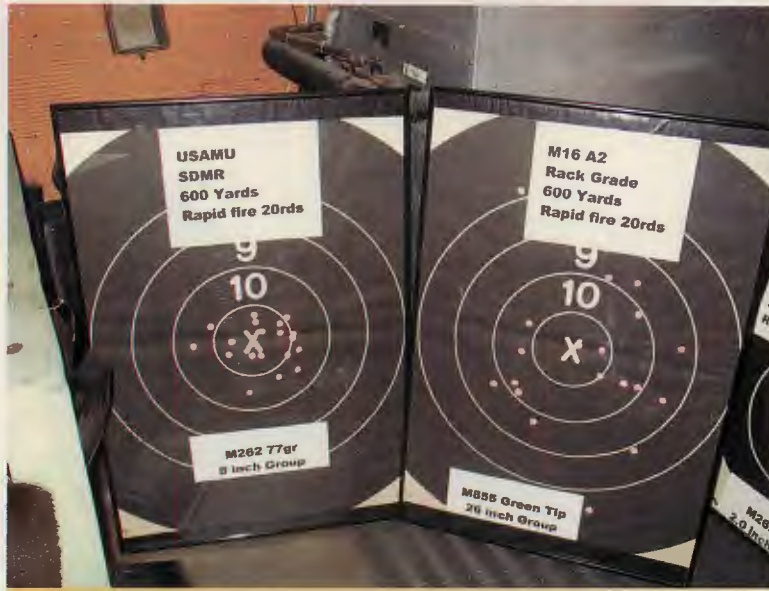
Representative targets show gain in accuracy potential of SDM rifle over one "off the rack" – a significant improvement.
